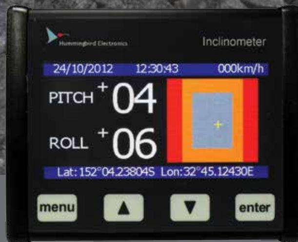
The Premium Inclinometer provides a full colour configurable pitch and roll display that is highly visible to operators of industrial machinery. Many aspects of the Inclinometer are customisable, including positioning and sensitivity of the sensors, separate alarms and warnings for stationary or moving vehicles and four distinct primary display options.
