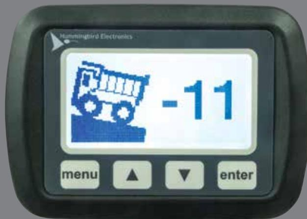
The Dual-Axis Inclinometer provides a highly visible and configurable pitch and roll display to operators of industrial machinery.
