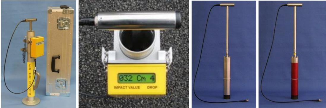
Features: Clear Anodised Aluminium Guide Tube, Aluminium-Clad Plywood Shipping Case, Stainless Steel T-Handle, Stainless Steel Hammer Weight for 4.5 kg Version or Red Anodised Aluminium Hammer Weight for 2.25 kg Version.
