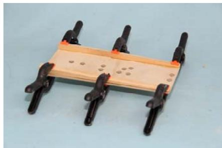
When the glue has dried paint all surfaces EXCEPT the tapered rail surfaces, (they should be kept as bare wood to obtain best adhesion with the epoxy glue when fitting to the hull) with the clear polyurethane varnish to be used when finishing the decking.
