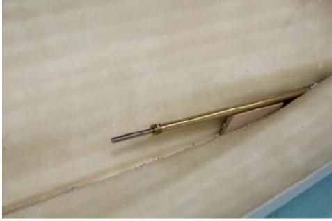
Take the propeller shaft wedge (P/N 1240) and insert it in the inside of the hull under the propeller shaft to check that it will properly support the shaft when it is linked to the engine. It will be glued in position in a later step. Make any adjustments to the propeller shaft hole to achieve the correct alignment of the drive train.
