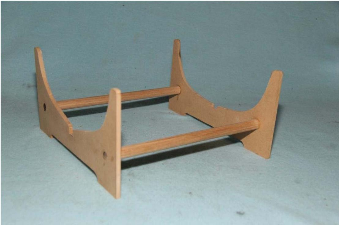
The four components comprising the boat stand assembly are illustrated above. Just apply PVA wood glue to the ends of the dowels and fit the end plates. Leave time for the glue to set and you are ready to start assembling your boat on the convenient platform you just made.
