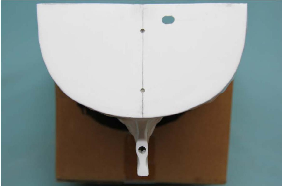
Trim the molding fin on the face of the skeg to provide a flat surface for drilling the hole for the propeller shaft (P/N 1265) as shown above. Mark a spot in the centre of the skeg face 25mm up from the bottom edge of the skeg.
