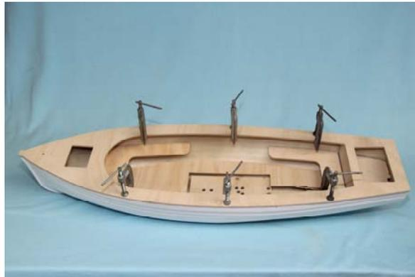
Since PVA glue is slow setting, it is possible to make adjustments to the connection after applying the glue but if not using clamps it is important to plan what you will do, and how, to maintain the desired position while the glue sets. If “holding it with your fingers while the glue sets” is the only option then epoxy glue should be used. By now you should have enough experience with epoxy to have an idea of how long you will have to hold on!
