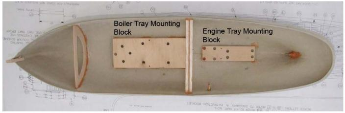
Position the Boiler Mounting Tray Block, oriented as shown above, and gently align it to the centreline of the hull with the rear end of the block square against the bulkhead. Place a mark on the hull 40mm from the after edge of the Boiler Block to establish the correct position of the Engine Tray Mounting Block as illustrated. Using Epoxy 2 Pack adhesive set the blocks in place and put aside to allow the adhesive to set.
