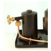
DO NOT EVER BE TEMPTED TO REFILL THE TANK WHILE IT IS IN POSI-TION IN THE BOAT—YOU RUN A SERIOUS RISK OF TRIGGERING AN EXPLOSION WHEN RESTARTING THE BOILER.
