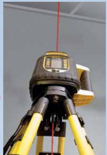
Plumb Up and Down. Laser dot using internal compensator.
