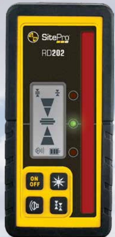
RD202 - Long Face - included 2 x LARGER 125mm Capture Window Front and back displays - range up to 700m IP56, LCD & LED, 1.0mm/2.5mm
